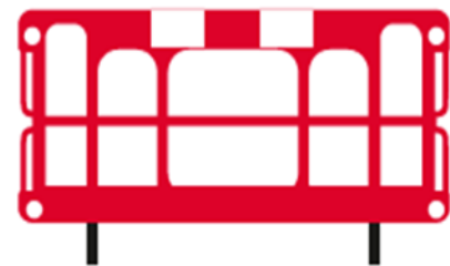
Typical pedestrian barrier with tapping rail
